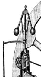
As the rotary speed of the governor declined, a series of operations served to control the steam engine. The valve gradually opened under the force of gravity, more steam was admitted, rotation increased, the revolving balls rose, the flow of steam declined, and the irregularities of the engine were smoothed out. Such feedback, that is, served to steady the working of the machine.
